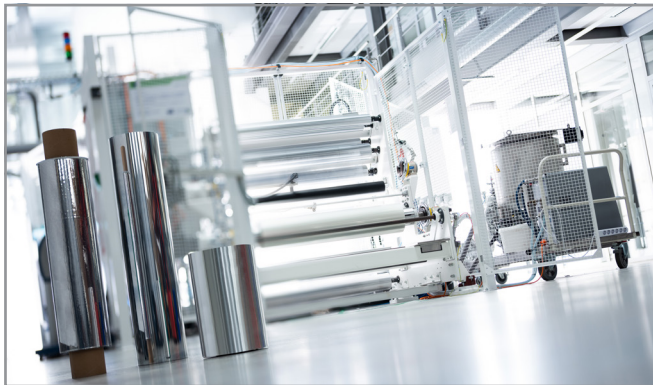
Roll-to-roll pilot coating line atmoFlex 1250 with 1200 mm coating width for the R2R-NIL process
