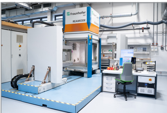
REAMODE – Test facility for the modification of organic materials with accelerated electrons
