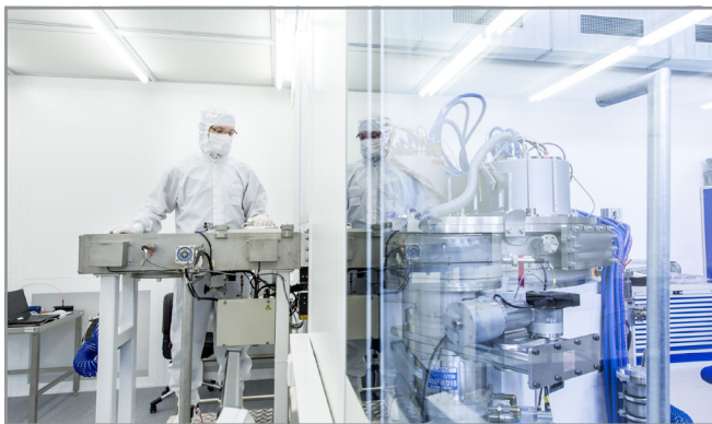
Cluster systems of the Fraunhofer FEP for pulse magnetron sputtering processes
