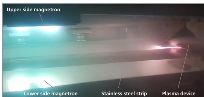
Experimental setup for catalyst coating and graphene synthesis
