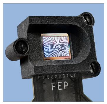
**High-resolution OLED-on-silicon fingerprint sensor** © Fraunhofer FEP | Picture in printable resolution: www.fep.fraunhofer.de/press
