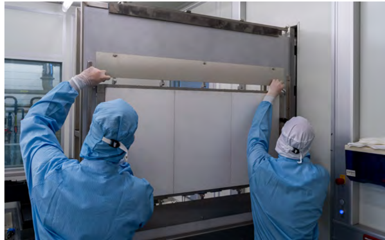
E-chuck transfer of the three-part electrostatic chuck system for 600 × 1200 mm 2 substrates onto the carrier of the vertical in-line coating system
