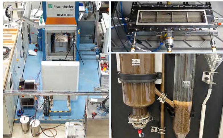
Integration of the ARA module for the combined treatment of liquids with low-energy electrons and ozone (top right) in the REAMODE laboratory plant (left). Simulation of the biodegradability of the transformation products in a laboratory wastewater treatment unit (bottom right).
