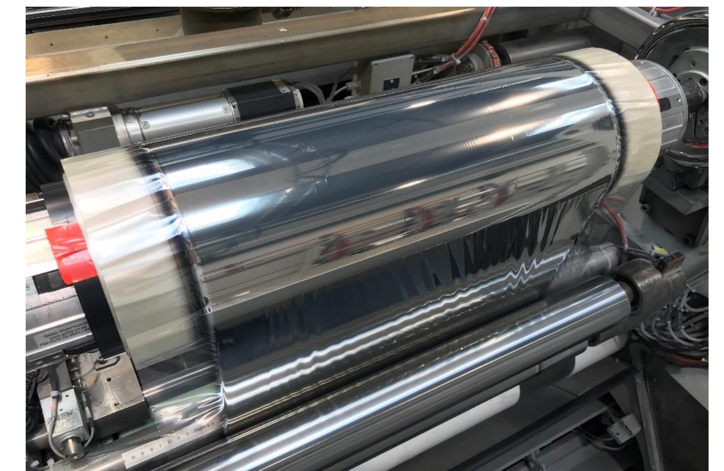
Wrinkle-free metal-on-polymer current collector coil after deposition. Coil width 650 mm
