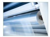
We develop technologies, processes and key components for the vacuum coating of flexible products such as polymer films and thin metal foils, textiles, membranes and paper. Surface refinement with thin layers enables these materials to be used in a variety of innovative products. A very effective, cost-efficient process for modifying the surfaces of flexible materials is vacuum web coating, so-called roll-to-roll processes.
